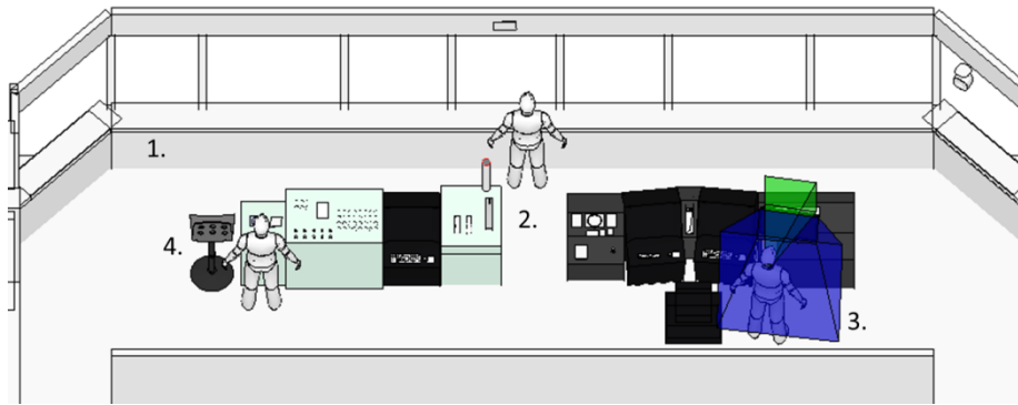
Figure 36: Visualization of the Use Case's Simulation Environment with its hull (1), human and machine agent body geometries (2), sensomotoric geometries (3) and artifacts (4)
