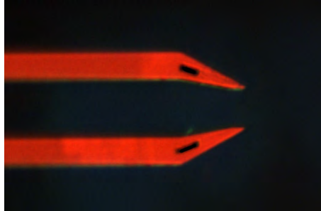
Figure 3.2: Micro gripper in a microhandling setup (Diederichs and Fatikow, 2012). If the gripper jaw is tracked, PCA based features are of great help.
