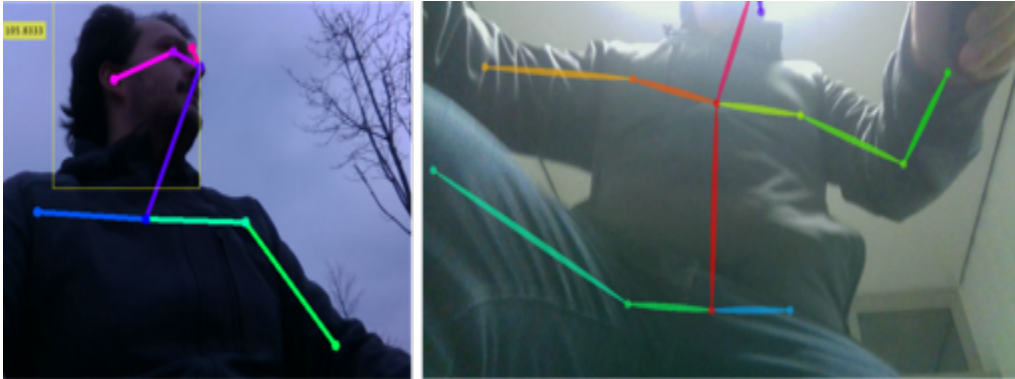
Figure 7.3: Recognition of head movement (left) and hand gestures (right) of cyclists using the OpenPose library.
