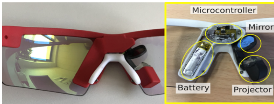
Figure 7.5: The HUD glasses and its components. The microcontroller is powered by the battery and connected to a projector. The projection is reflected by the mirror and seen in the front.
