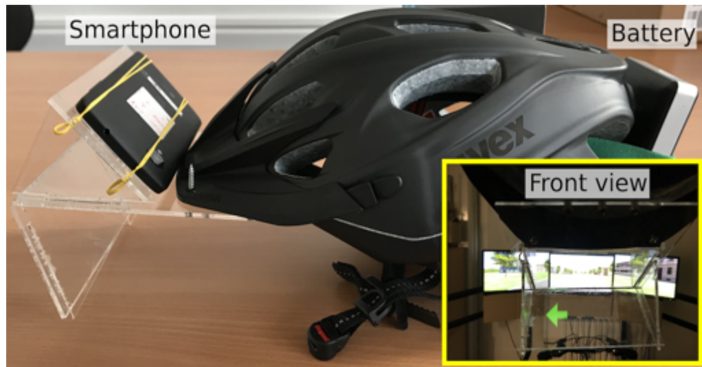
Figure 6.6: HUD helmet: visual cues displayed on the smartphone were reflected in the plexiglas surface of a holder in the front. A battery power bank at the back was used to balance the weight and change the smartphone.
