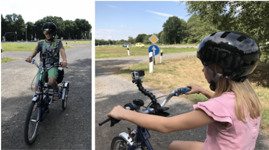
Figure 5.1: A mid-size tricycle and helmets equipped with auditory, light and vibrotactile navigational cues for investigation in an outdoor practice test track.
