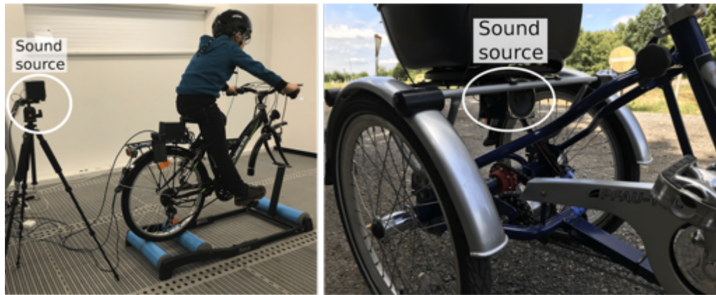
Figure 5.5: Setup for the auditory distraction task used in the lab (left) and controlled test-track (right) experiments. The sound source in the lab study was mounted on a tripod behind the bicycle. In the test-track study the sound source was mounted on the frame of the bike behind the seat.
