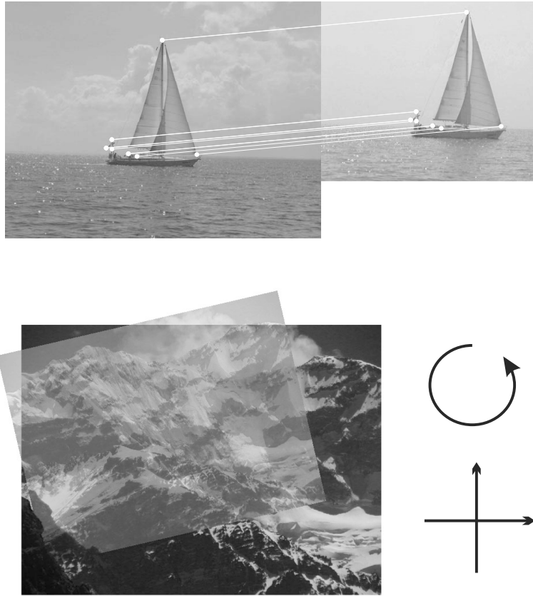
Figure 3.1: Basic types of image registration strategies. The upper image shows corresponding pairs of features which are used to derive transformation model parameters (feature-based registration). In the lower image, two views of an image scene are registered by iteratively modifying the transformation model parameters and evaluating a similarity measure (area-based registration).
