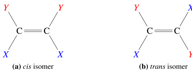
Figure 4.15: This is an example of a molecule with one cis and one trans isomer. Because of the double bond between the carbon atoms, they cannot rotate freely and all six atoms are coplanar, meaning they are in the same plane. X and Y can represent different single atoms or groups of atoms, e.g., for butene X = \text{CH}_3 and Y = \text{H} . For the cis isomer, the groups are on the same side (a) and for trans on opposite sides (b).
