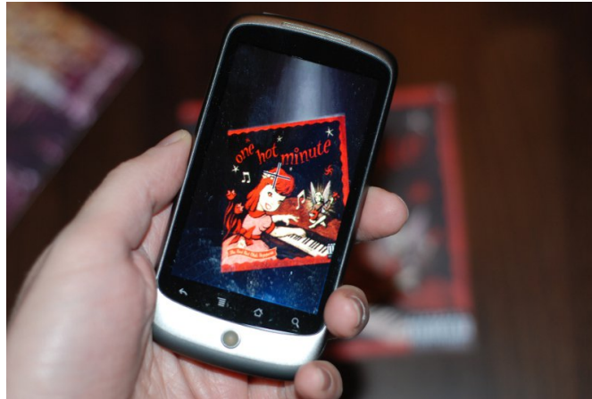
Figure 4.23: The two-step interface that shows no information or playback controls on the screen. The object is highlighted by displaying a coloured image of the CD on top of a greyed out background. The user has to select the CD to go to another view that provides information and playback controls.
