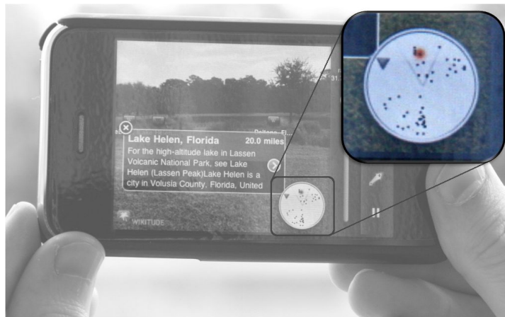
Figure 5.12: The off-screen visualization of the Android version of Laya. Laya displays nearby POIs using a mini-map.
