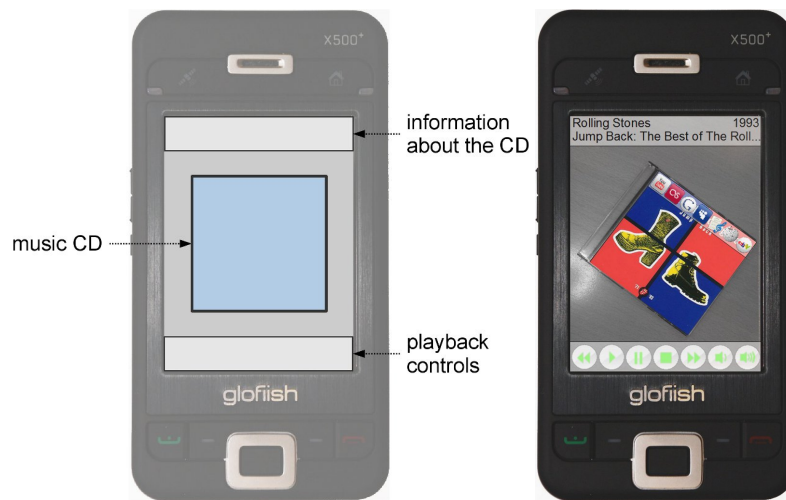
Figure 4.10: Concept and mock-up of the phone-aligned interface to augment music CDs. The design aligns the buttons to control music playback to the display's bottom and information about the CD to the display's top.
