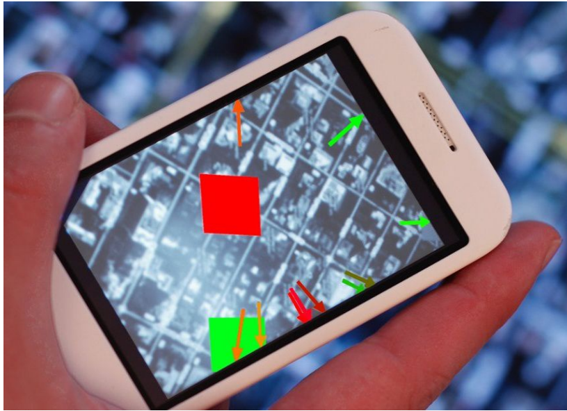
Figure 5.8: Physical map augmented using a mobile phone. POIs on the map are shown with coloured rectangles and arrows pointing at object beyond the display.
