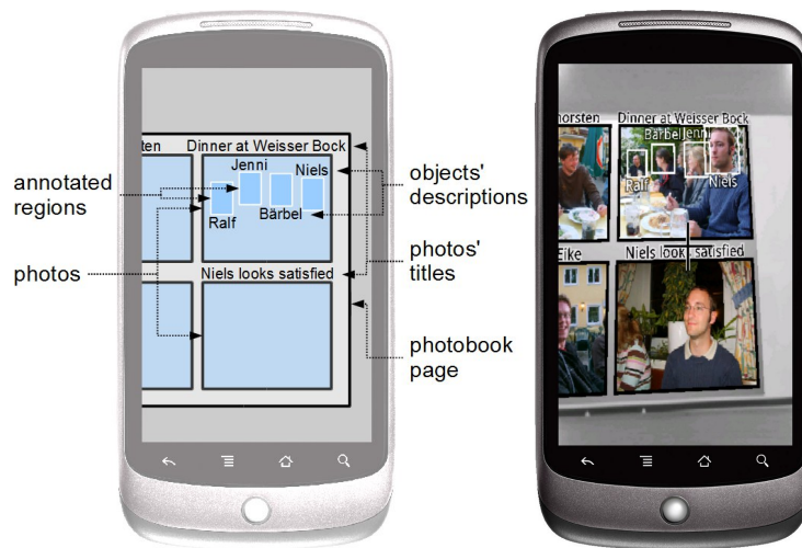
Figure 4.7: Concept and mock-up of the object-aligned interface to augment photo books. The design aligns the annotations to the photos and thus the annotation is visible for all photos simultaneously.
