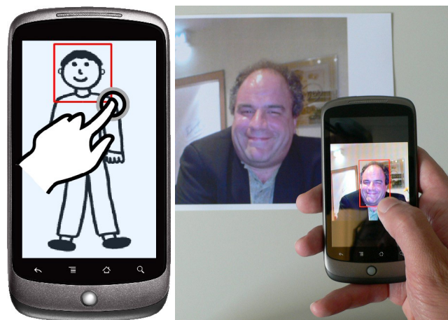
Figure 4.14: The interaction technique to select regions of photos that uses a static picture.
