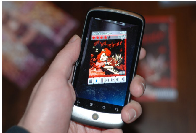
Figure 4.21: The object-aligned interface that aligns the information and playback controls to the CD's top and bottom. The object is highlighted by displaying a coloured image of the CD on top of a greyed out background.
