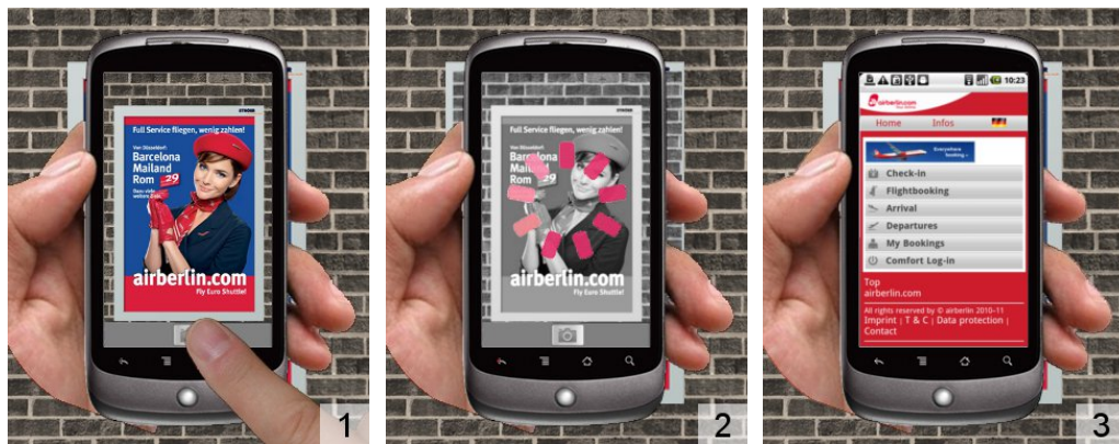
Figure 3.2: The interaction flow using Point & Shoot. After spotting an advertisement poster and starting the application the user aims at the poster (1). The user takes a photo that is analysed (2) and receives the according website if the poster has been recognized (3).
