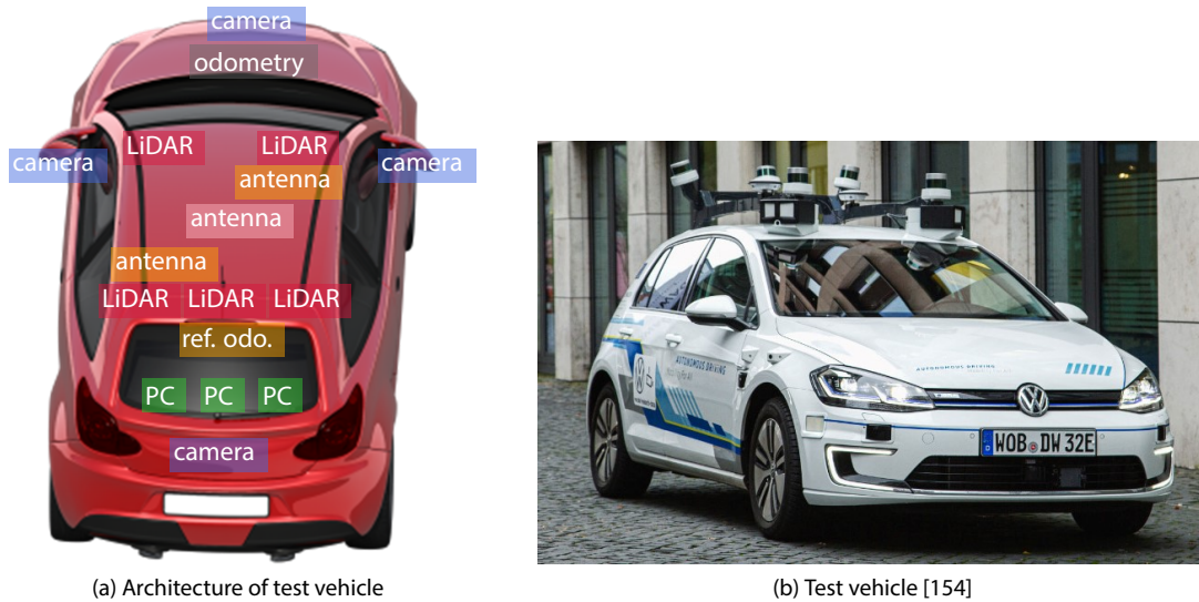
Figure 3.1: Sensor setup, architecture, and image of the test vehicles with five LiDAR sensors (red), four cameras (blue), a low-cost GPS (pink antenna), a localization reference system with two antennas (orange), three PCs (green), and an odometry module (gray).
