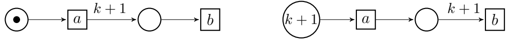
Figure 2.14: Petri nets solving sequences ab^{k+1} (l.h.s) and a^{k+1}b (r.h.s.) for k \geq 0 .
