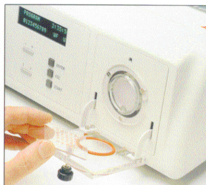
Inserting the grid support plate into the staining chamber
