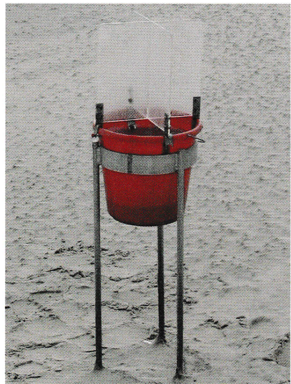
Fig. 2: Design of the coloured pan trap modified by the addition of an acrylic "windshield trap" (see text for further explanation).
