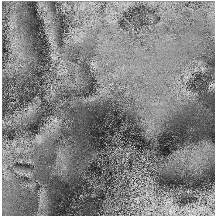
Figure 6: Phase difference modulo 2\pi representing deformations during time period of 4 minutes at 85% RH. Several sub-areas deform independently.
