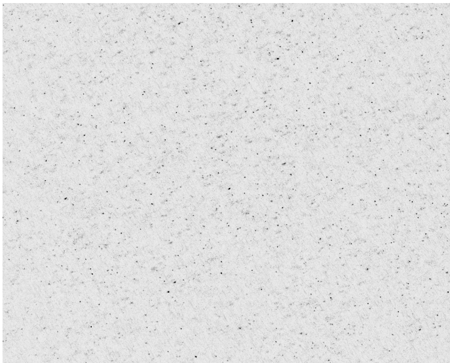
Fig. 11. Inverted image of a digitized plane ( 1280\text{ px} \times 1024\text{ px} ) from a reconstructed real image of a wind tunnel flow (DEHS particles after one hour of operation of the seeding generator). The image was obtained by an exposure time of 0,5 seconds, the field of view is 8,6 \times 6,9\text{ mm}^2 .
