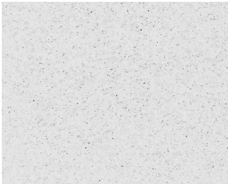
Fig. 7. Inverted image of a digitized plane (1280 px \times 1024 px) from a reconstructed real image of a wind tunnel flow (DEHS particles after one hour of operation of the seeding generator). The image was obtained by an exposure time of 0,5 seconds, the field of view is 8,6 \times 6,9 mm 2 .
