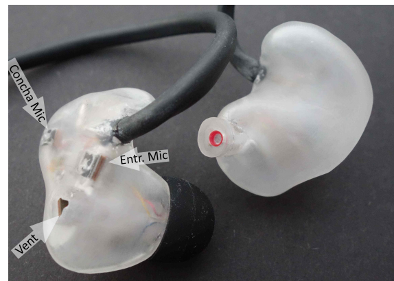
Fig. 3: Photograph of a right device, outside (left) and inside (right) view. The Entrance and Concha microphones are visible through the transparent acrylic, as well as the Outer Vent microphone inside the vent.
