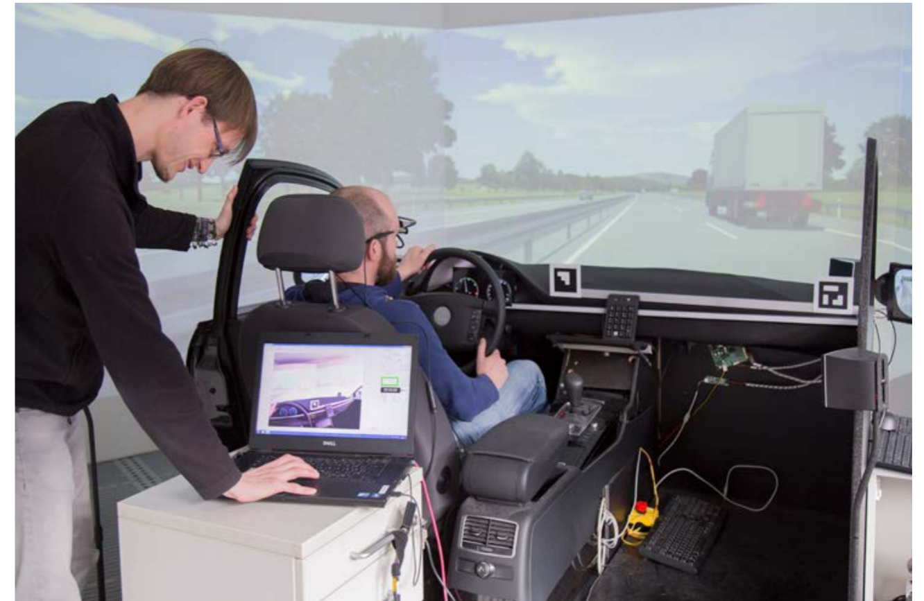
Scientists at Oldenburg University can test assistance functions for self-driving cars in the University's driving simulator.
